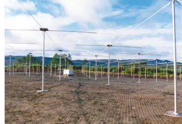
IRIS imaging riometer in Kilpisjärvi, Finland
