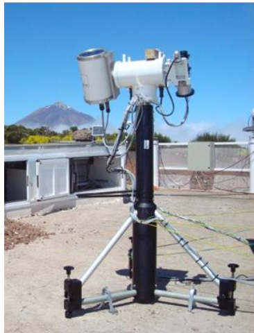
Figure 39: Left: the solar tracker and entrance optics during the solar measurements at Izaña. Right: comparison between SOLAR SOLSPEC, SIM (adjusted on ATLAS 3) and the ground-based validation.
