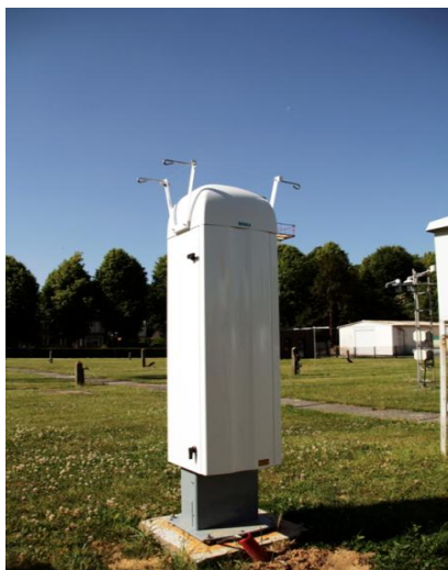
Figure 70: Lidar Ceilometer installed in Uccle
