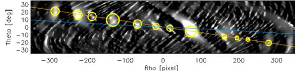
Fig.8: Hough space  $H_M(\rho, \theta) = \max_a H(\rho, a, \theta)$  for  $a = 1.1..10$ .
