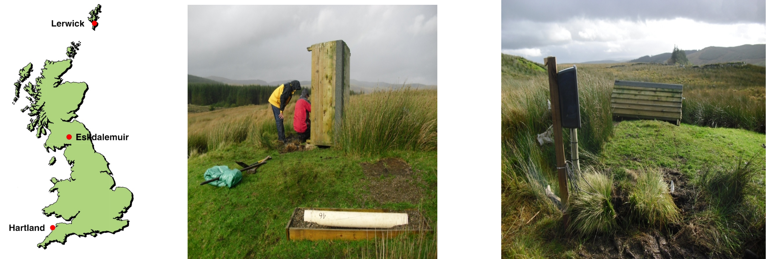
Figure 1: Left: Location of Eskdalemuir [55.314° N, 356.794° E] in the Scottish Borders, UK. Centre: The coils (white tube, foreground) are located in a rural valley (background), protected from wind, rain and snow under a non-magnetic wooden cover (shown upright in midground). Right: Looking eastward to the enclosed coil under wooden cover. The signal is digitized close to the coil before being converted to a higher voltage at a breakout box and sent to a logging computer in a vault approximately 150m away to the south.
