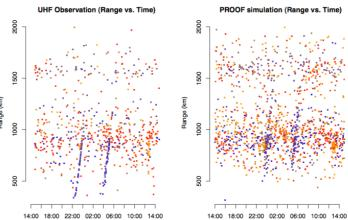
Comparison between measurements of the space debris environment as observed by the EISCAT UHF radar (left) and the predictions of the ESA PROOF model (right) (Markkanen et al, 2009). The clouds of vertically-distributed points correspond to debris fragments from the Cosmos-Iridium collision.
