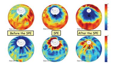
Variations in ozone density (top) and nitric oxide density (bottom) at 46 km altitude, as observed by the GOMOS instrument on ENVISAT, following the intense solar particle events (SPEs) during the Halloween superstorm of 2003 (Seppälä et al., 2004).
