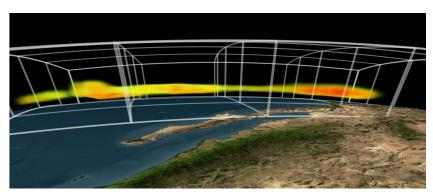
Schematic representation showing the volumetric imaging of an ionospheric layer by EISCAT\_3D.
