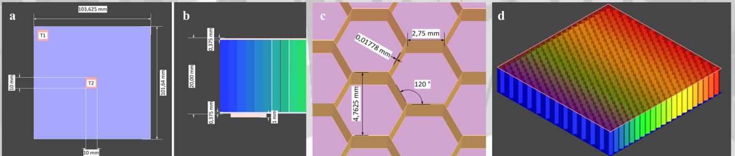
Figure 1: a,b) Measures of the analysed panel including the two silicon targets, c) the honeycomb structure and d) a view on the complete model.
