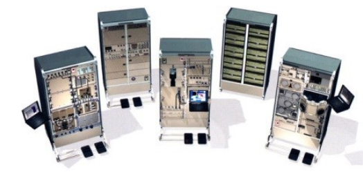
Columbus five internal payload racks at launch (courtesy ESA)
