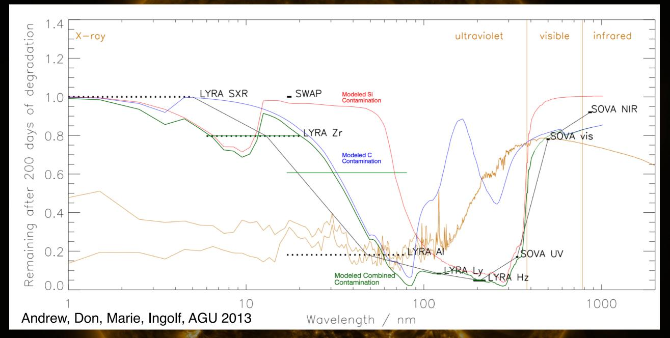
~ 13 nm of Si & C contaminants give a good fit for all channels except for the Al channel.
