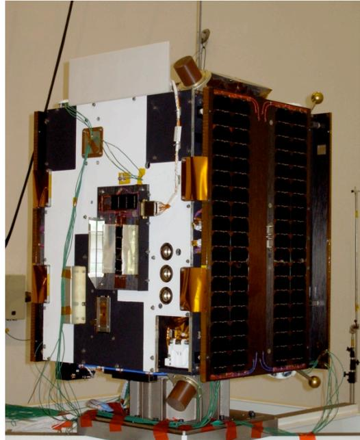
Figure 2 LYRA and SWAP after integration on the satellite. The three circles are the three eyes of LYRA. The rectangular opening under LYRA, gives a view on SWAP.
