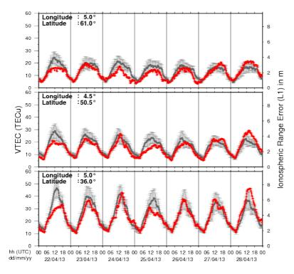
The figure shows the time evolution of the Vertical Total Electron Content (VTEC) (in red) during the last week at three locations:
