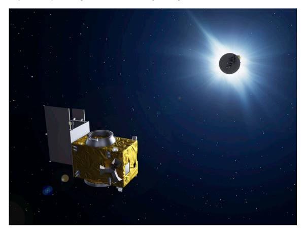
PROBA-3 is the ultimate state-of-the-art eclipse-producing machine guaranteeing exciting research of the solar atmosphere. An eclipse- maker is called a coronagraph. This coronagraph listens to the name ASPIICS.
