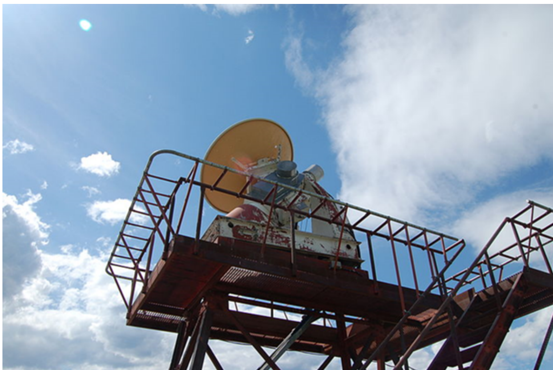
One of two Dominion Radio Astrophysical Observatory 10.7cm solar flux monitoring telescopes. Taken 02 July 2007 by Jason Nishiyama. Wikimedia Creative Commons Attribution-Share Alike 3.0 Unported license
