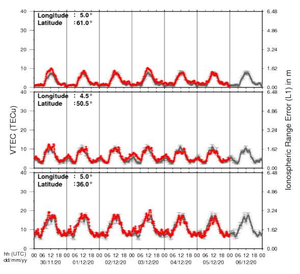
The figure shows the time evolution of the Vertical Total Electron Content (VTEC) (in red) during the last week at three locations:
