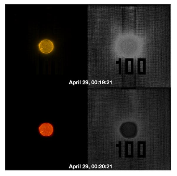
At first glance, as pretty as these images are, they look like what we expect. But by cleverly making use of a feature that is typically used to help calibrate the images on-board, the EUI team commanded their instrument to include a watermark inside these two images. When filtering these images for vertical features, the watermark '100' clearly becomes visible.
