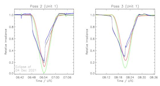
The occultations were also observed by LYRA's "calibration unit" (unit 1) in addition to the nominal one (unit 2). The plots above show normalized observations by LYRA during two passes in the eclipse zone. The colors correspond to the observations by the four channels of LYRA: red = Lyman-alpha, green = Herzberg, blue = Aluminum, black = Zirconium.
