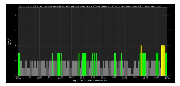
Local K-type magnetic activity index for Belgium based on data from Dourbes (DOU) and Manhay (MAB). Comparing the data from both measurement stations allows to reliably remove outliers from the magnetic data. At the same time the operational service availability is improved: whenever data from one observatory is not available, the single-station index obtained from the other can be used as a fallback system.
