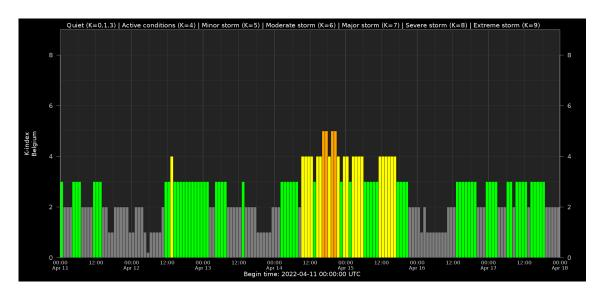
Local K-type magnetic activity index for Belgium based on data from Dourbes (DOU) and Manhay (MAB). Comparing the data from both measurement stations allows to reliably remove outliers from the magnetic data. At the same time the operational service availability is improved: whenever data from one observatory is not available, the single-station index obtained from the other can be used as a fallback system.
