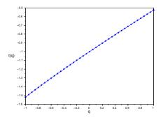
$\tau$  function associated to the previous signal. Linear regression gives a slope of 0.494021.
